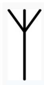
This is the accepted symbol for an antenna
