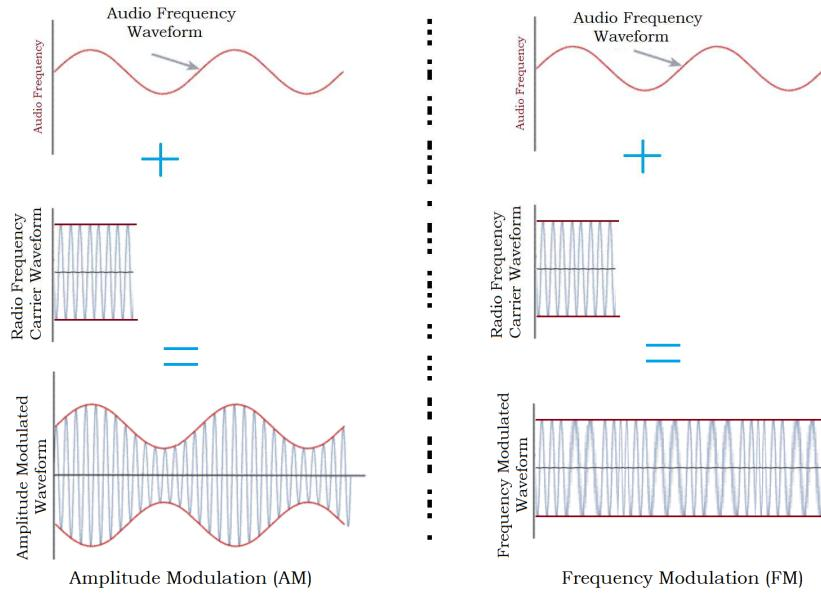
The location of where differing (audio, radio and modulated) waveforms occur in a simple transmitter.
