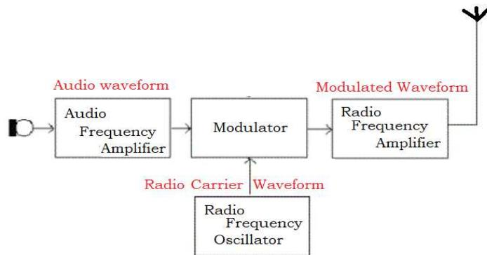
A transmitter is designed for a **specific impedance** at its antenna socket. If it does not "see" this impedance then the PA (Power amplifier) cannot operate efficiently. The usual impedance of a feeder for coax is **50 ohms**. An antenna will only present an impedance near to 50 ohms when it is the correct size for the applied frequency. A BALUN (or UNUN) can be used to match the impedance to that of the transmitter (see Module 3 for more on antennas).
