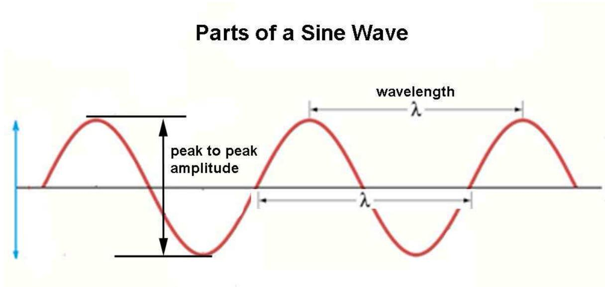
In a simple radio wave, the intensity of the electric and magnetic fields oscillate (they change direction smoothly) at a particular frequency.
