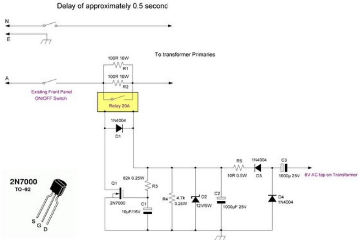
3. Here is a schematic of an easy to build PTT interface for the TL922.
