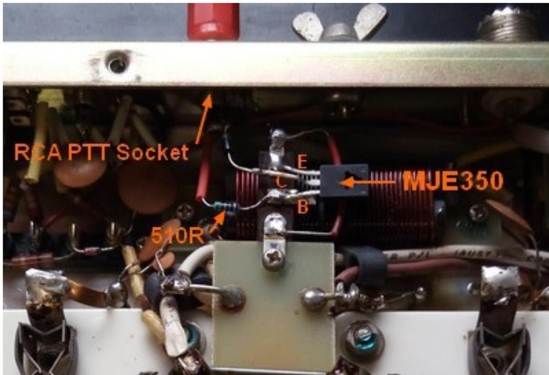
4. The last modification - a mandatory one where a tetrode is going to be retrofitted in lieu of the 3-500Z, is to ground all grid pins on the sockets directly to chassis. The silver mica capacitors installed during the factory build can be removed, and if in good electrical and physical condition may be useful for other projects requiring capacitors to carry RF currents.
