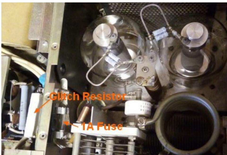
Note the hairpin anode parasitic suppressors fitted to the tubes. They were part of previous modifications and are generally accepted to be more broadband in their operation than the traditional coiled choke.
