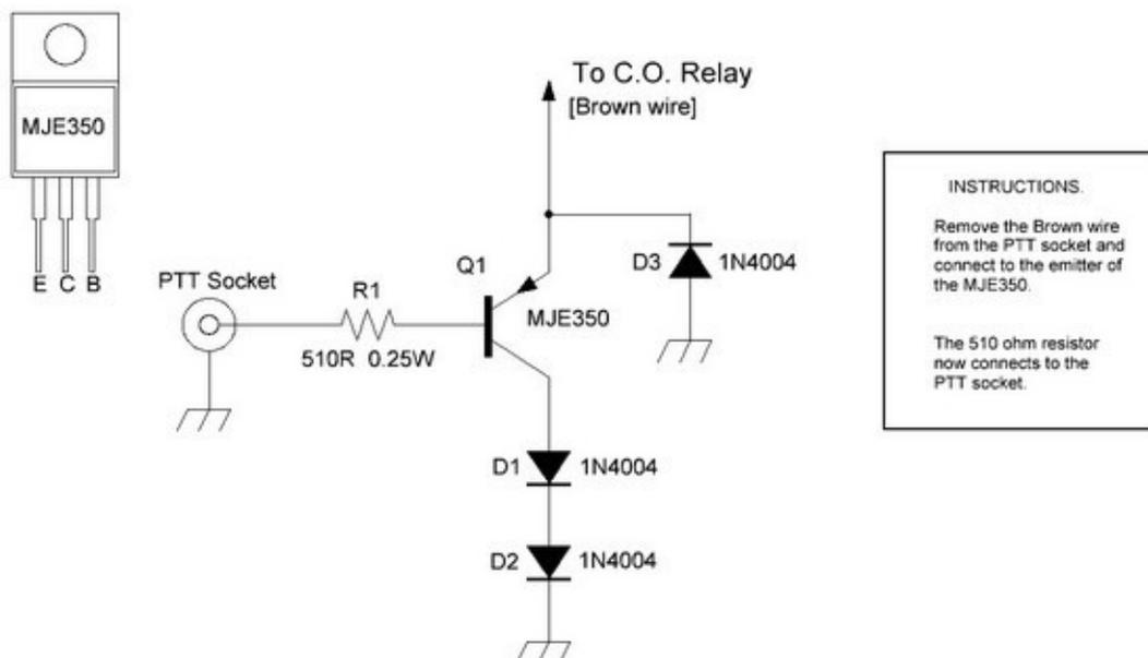
When the TL922 came onto the market in the late 1970s many transceivers had tube finals and PTT switching relays that could handle the 100V or more from the amplifier keying line. To interface with modern rigs, often an external relay or robust solid state circuit protected the rig from high keying line voltages. My design is extremely simple but effective and is wired on a mini-tag strip close to the RCA PTT socket on the amplifier as per this photograph.
