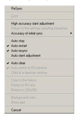
**ReSync** - Clicking this will resync the picture if the sync sign was lost or interrupted for a second.
