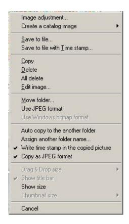
**Image Adjustment** - Clicking this will bring up a image adjustment window, where you can control the brightness, hue, contrast etc. clicking on the edit button will bring the MS paint program to further edit your image.
