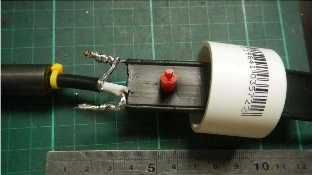
The last photo shows my completed second antenna. Note how I have cable-tied the coax to the side of the balun to prevent strain on the point where it exits the balun.
