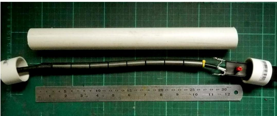
This photo shows how it is constructed. Again, HP pipe and caps (25mm) are used. You might be able to get away with 20mm diameter, however you are limited by the width of the window line. The ferrite beads are prevented from moving by small cable ties at each end. The left (output) end is
