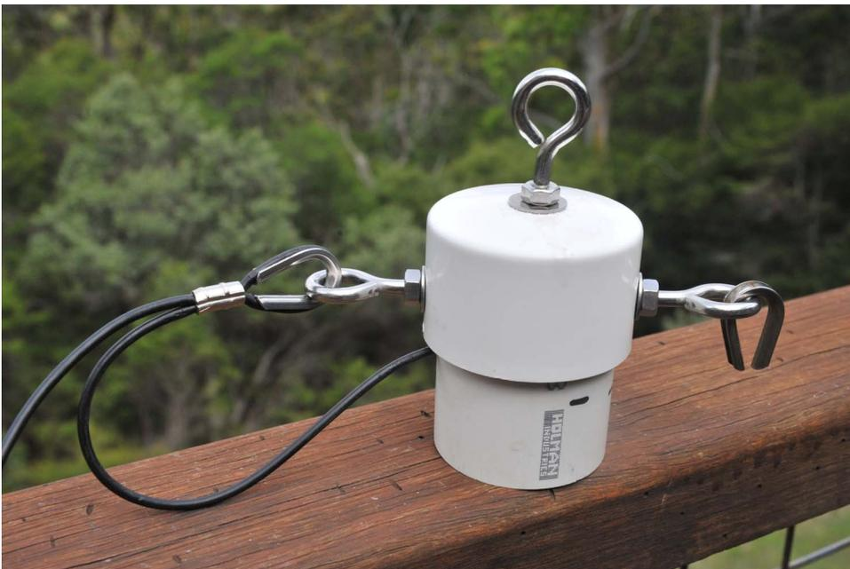
In the antenna shown above, I used 14 AWG insulated hi-flex wire from Davis RF.
